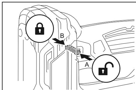
To prevent the switch trigger from accidentally pulled, the trigger-lock button is provided.
