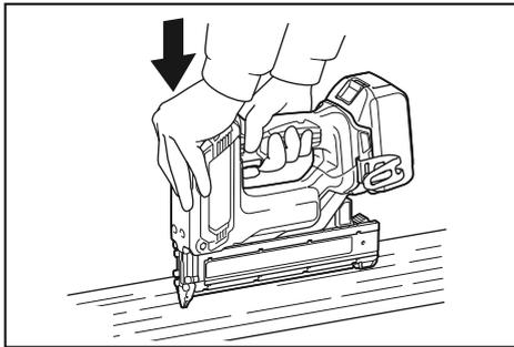
**NOTE:** If the head of the nail still remains above the workpiece even you hold the nail head, the material may not be suitable for the nailer. Continuing to use the nailer on such material may result in a damage to the driver of the nailer and/or nailer jamming.
