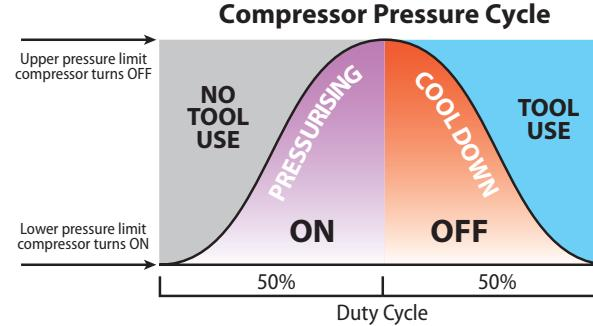
Compressing air produces heat which can damage the compressor if it's not managed. When the compressor turns off (after reaching maximum tank pressure) it has time to cool down while the air in the tank is being consumed.
